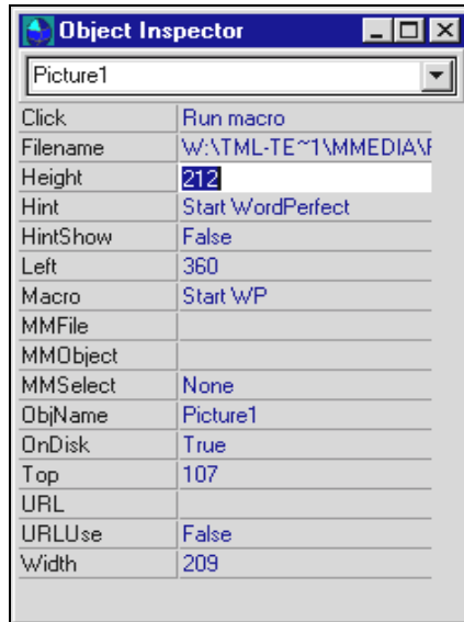
Figure 6.14: The Object Inspector showing picture properties.
