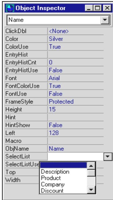
Figure 6.32: Associate the Selection List with an edit field from the Object Inspector.
